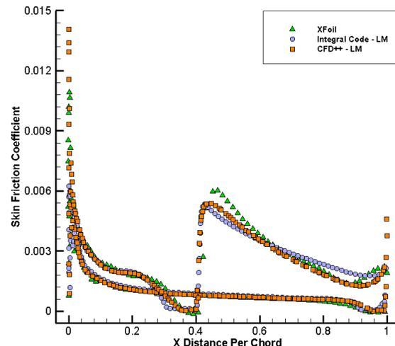
**Figure 4. Skin friction. CFD++ LM input to integral code compared to CFD++ LM and Xfoil.**
